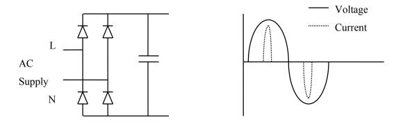
Distorted current waveforms are undesirable because they can lead to several problems in the ac supply. Examples include: reduction of power factor, causing excessive heat losses in the transmission cables, and excessive neutral currents in balanced three phase systems; and distortion of the supply voltage, which may interfere with other equipment using the same supply.
