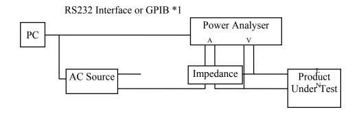
\*1: An RS232 to GPIB converter will be needed for GPIB control of the PM6000.
