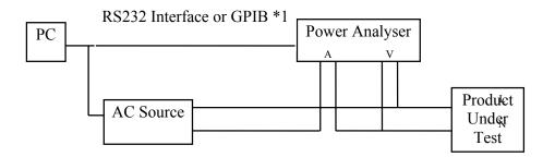
\*1: An RS232 to GPIB converter will be needed for GPIB control of the PM6000.
