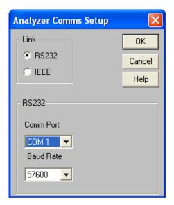
Having set up the communications interface for the Power Analyzer, clicking OK will return you to the Top Level menu. (This obviously
