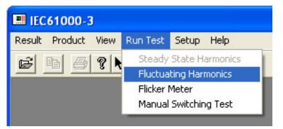
and the software will automatically configure the analyzer and AC Source.
