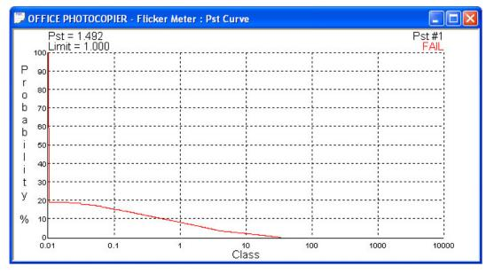
There will be a series of Pst curves - one for each ten-minute period in the measurement. You may view each curve in turn by using the < and > keys to scroll through the series.
